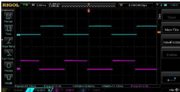
Fig. 14: Output of Inverter Switching Pulses
