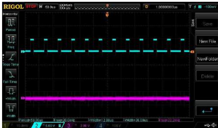
Fig. 13: Output of Boost Mode Pulses Buck Off
