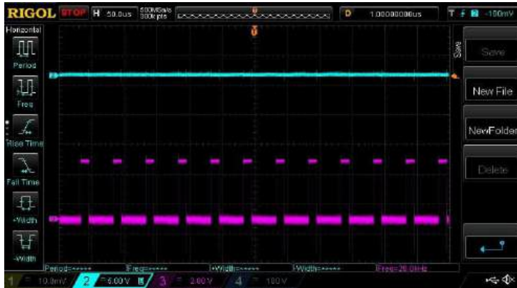
Fig 12: Output of Buck Mode Pulses Boost Off
